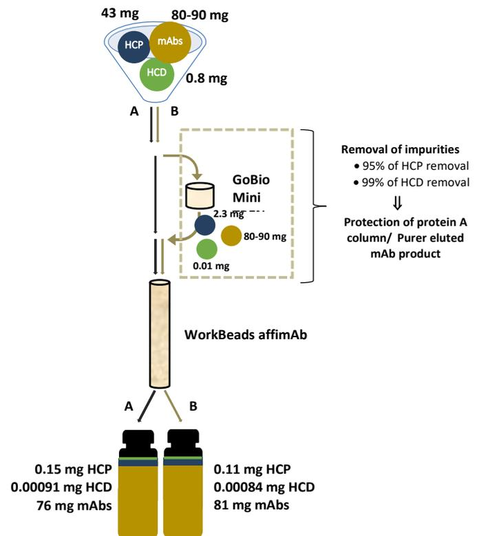
**Figure 8.** An illustration of reduction of impurities by using WorkBeads 40 TREN for pre-treatment upstream of the WorkBeads affimAb column at a heavy sample load. (A) Direct load of the CHO sample onto the protein A column, (B) Loading via pretreatment. Yellow: mAbs, blue: HCP, and green: HCD.
