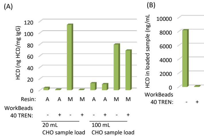
**Figure 6.** (A) HCD analyses of the collected mAb eluates. A: WorkBeads affimAb, M: MabSelect SuRe. The values are presented in ppm levels (ng HCP or ng HCP/mg eluted IgG). (B) HCD level measurements of flow-through of CHO cell supernatant, with and without WorkBeads 40 TREN.
