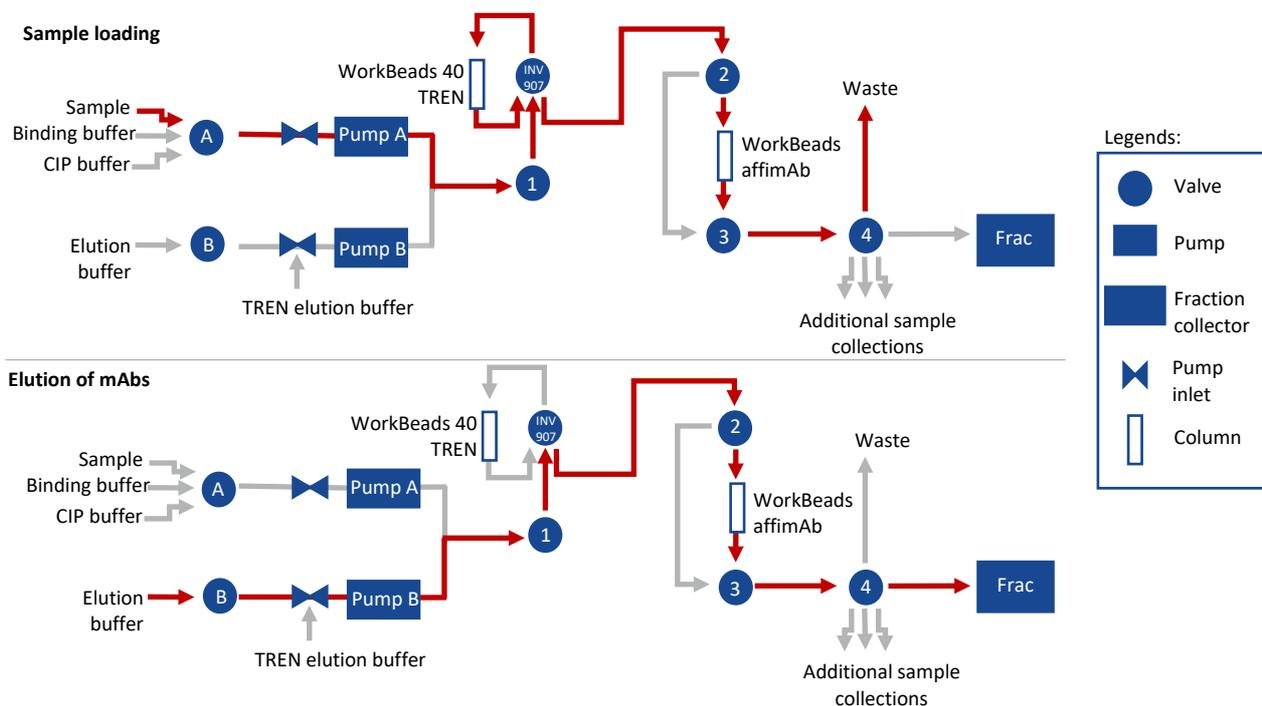
**Figure 2.** Flow chart of the purification method in which WorkBeads 40 TREN is acting as a pretreatment resin before WorkBeads affimAb. The GoBio Mini TREN column is positioned in Valve INV-907, position 2, and WorkBeads affimAb is positioned between valves 2 and 3. The top flow chart illustrates the flow during sample loading (red arrows) and the bottom flow chart illustrates the flow during the elution of mAbs (red arrows). Other steps in the process are not shown.
