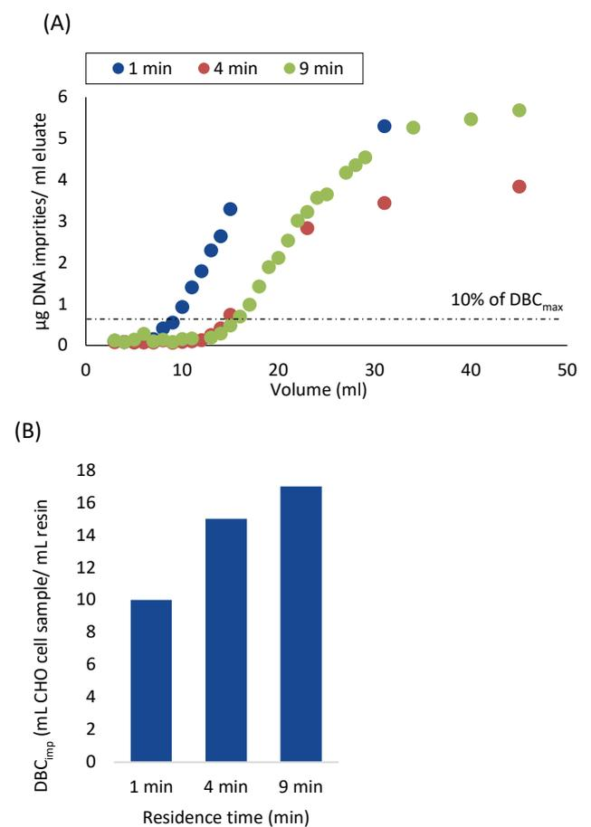
**Figure 7.** (A) Frontal analysis determination of dynamic binding capacity. (B) Measured  $DBC_{imp}$  at a residence time of 1, 4 and 9 minutes in a 7 x 28-mm column (GoBio Mini TREN 1 mL).
