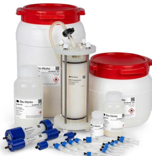
**GoBio Mini IEX Screening kit for easy screening to find optimal running conditions includes one GoBio Mini 1 mL column of each of the four ion exchangers. GoBio Mini Peptide Purification kit is a bundle of GoBio Mini S 1 mL and GoBio Mini Q 1 mL.**
