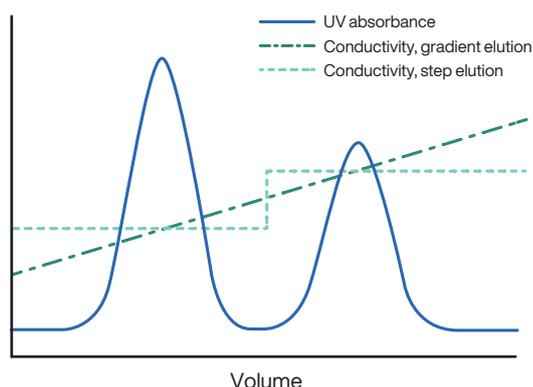
**Figure 3.** Optimization of step elution with salt. A test run with linear gradient elution gives information about suitable salt concentrations to be used in step elution. Note: Remember to take the system dead volume into account when comparing the gradient and the trace.
