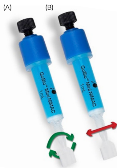
Figure 1. Removal of the cut-off end at the column outlet should be done by cutting or by twisting (A), not bending (B).
