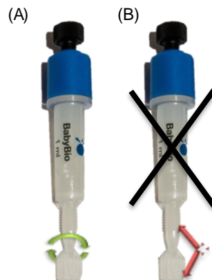
Figure 2. Removal of the cut-off end at the column outlet should be done by cutting or by twisting (A) not bending (B).
