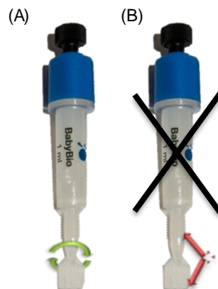
Figure 3. Removal of the cut-off end at the column outlet should be done by cutting or by twisting (A) not bending (B).
