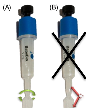
Figure 2. Removal of the cut-off end at the column outlet should be done by cutting or by twisting (A) not bending (B).
