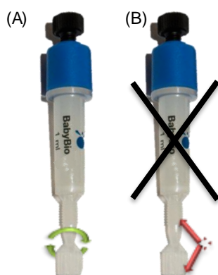
Figure 2. Removal of the cut-off end at the column outlet should be done by cutting or by twisting (A) not bending (B).
