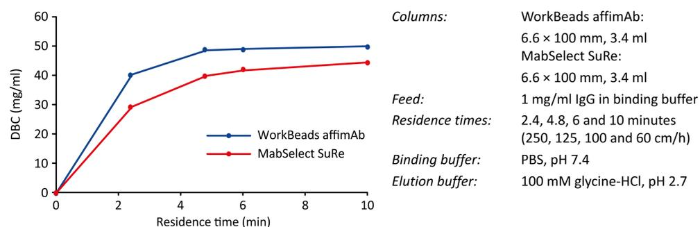
Figure 1. DBC for human polyclonal IgG determined at different flow rates (residence times) by frontal analysis on WorkBeads affimAb (blue) and MabSelect SuRe (red).
