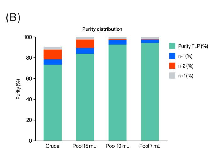
(A) PS ON elution pattern on AIEX. 20 mg PS ON crude was purified per mL WorkBeads 40Q resin. Elution buffer gradient (green), UV traces 260 nm (blue), and 295 nm (orange). Green boxes represent collected pools. (B) PS ON purity distribution within the crude, and each pool, for the resolved species: FLP (green), n-1 (blue), n-2 (red) and n+1 (grey) using RPC analysis.
