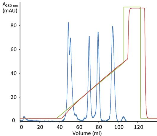
Figure 2. Separation on a cation exchange chromatography column of, peaks from left to right, concanavalin A,  $\alpha$ -chymotrypsinogen A, ribonuclease A and lysozyme. A 1-ml sample was applied onto WorkBeads 40S column, 100 mm bed height. The blue line corresponds to the absorbance at 280 nm, the red line to the conductivity and the green line to the percentage of the elution buffer.
