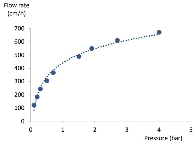
Figure 4. Pressure to flow rate properties of WorkBeads 40S determined with deionized water, 25 x 200-mm glass column.
