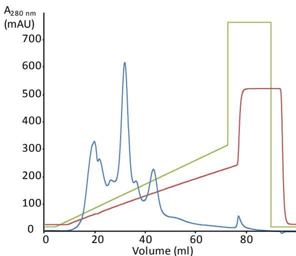
Figure 3. Separation on anion exchange chromatography column of, peaks from left to right, apo-transferrin,  $\alpha$ -lactalbumin and soybean trypsin inhibitor. 10 ml sample applied onto a column packed with WorkBeads 40Q resin. 100 mm bed height. The blue line corresponds to the absorbance at 280 nm, the red line to the conductivity and the green line to the percentage of the elution buffer.
