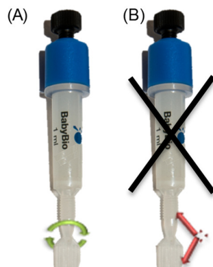
Figure 1. Removal of the cut-off end at the column outlet should be done by cutting or by twisting (A) not bending (B).
