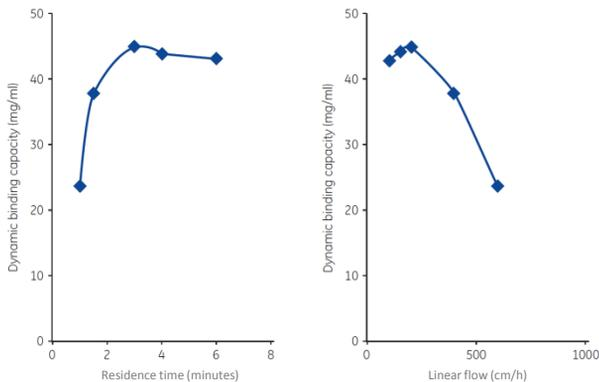
Figure 1. Effect of residence time and linear flow on dynamic binding capacity.
