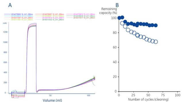
Figure 3. Alkaline stability of WorkBeads Protein A. A) Frontal analysis. B) Remaining DBC after CIP cycles using 15 mM NaOH (closed circles) or 100 mM NaOH (open circles).
