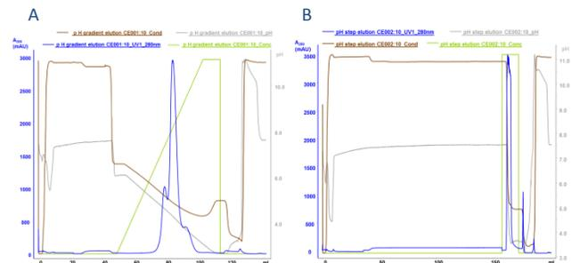
Figure 2. Binding and elution of human polyclonal IgG on WorkBeads Protein A. A) pH gradient elution pH 5.6-2.1, B) Step elution at pH 3.2
