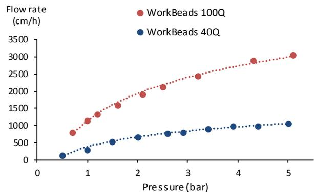
Figure 4. Pressure-flow properties of WorkBeads 100Q and WorkBeads 40Q. The data was obtained using distilled water passed through a 10 mm (i.d.)  $\times$  200 mm bed of resin in a glass column. The bed was open, i.e., the top adaptor was not pushed towards the chromatography bed.
