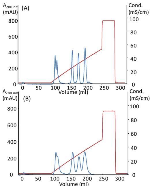
Figure 3. Chromatogram of selectivity on two different cation exchange resins, WorkBeads 40S (A) and WorkBeads 100S (B).
