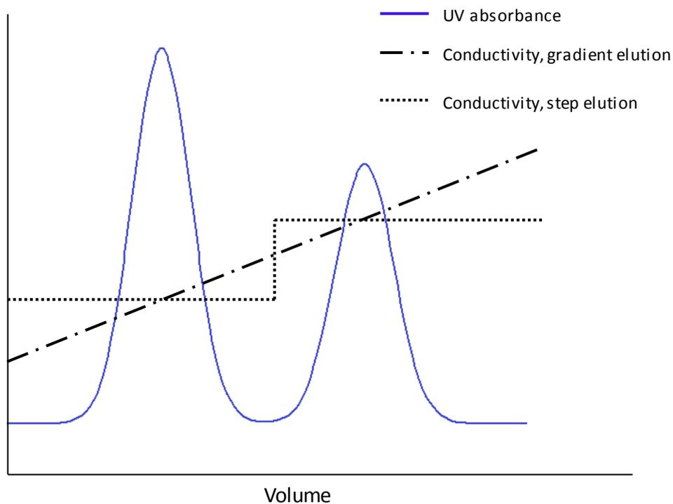
Figure 2. Optimization of step elution with salt. A test run with linear gradient elution gives information about suitable salt concentrations to be used in step elution. **Note:** Remember to take the system dead volume into account when comparing the print out of the gradient and the trace.
