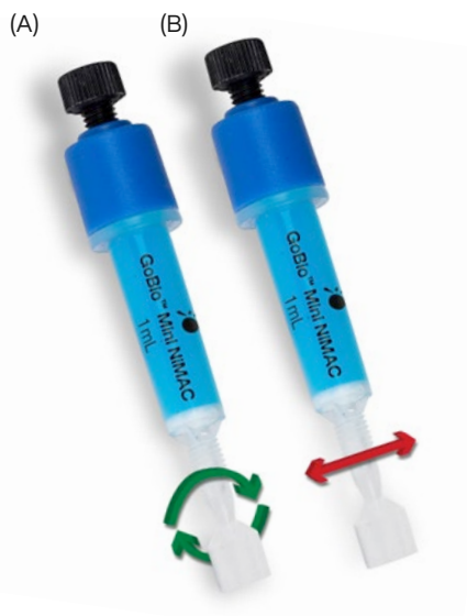
Figure 1. Removal of the cut-off end at the column outlet should be done by cutting or by twisting (A), not bending (B).
